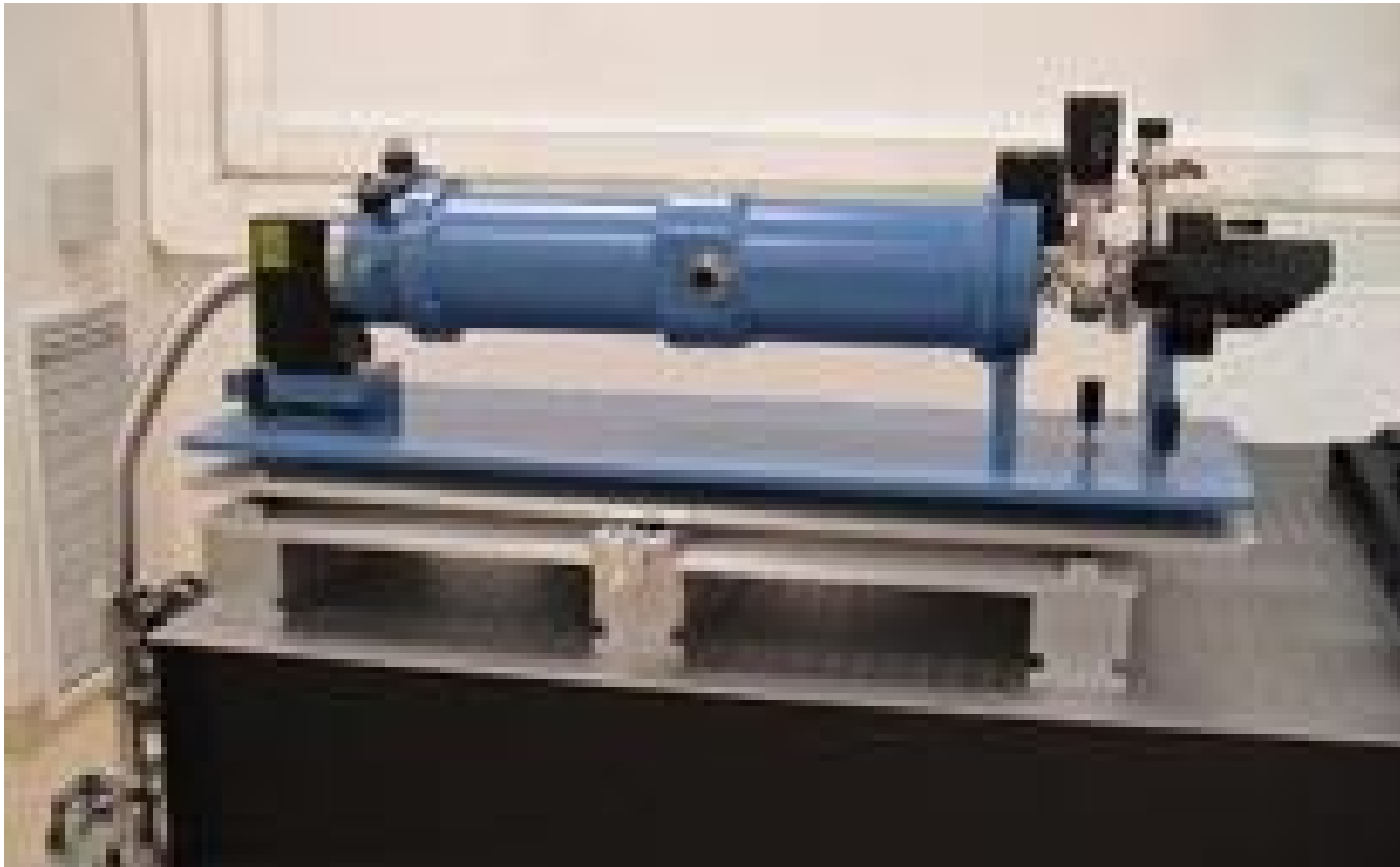
UK National Physics Laboratories (NPL) Primary Standard cryogenic radiometer
