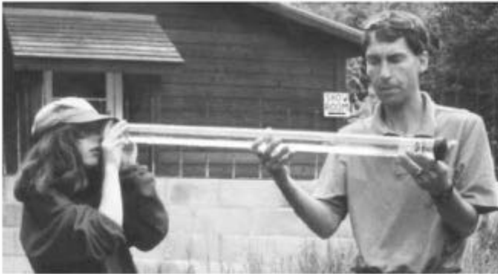
Fig. 1 SHMAK clarity tube for measuring water clarity. (Photo: Helen Ricketts.)
