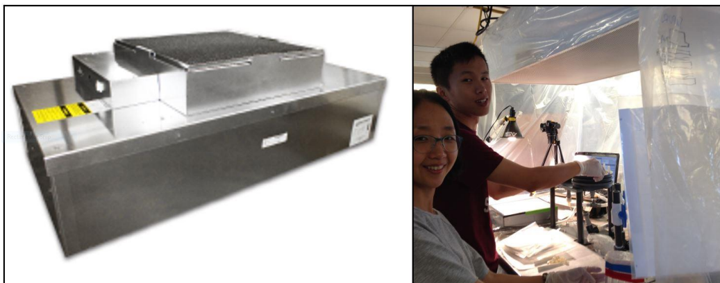
Figure 3. Left: MAC 10@ LEAC 2x4 ft (600x1210 mm) fan filter unit (Enviroco, Sanford, NC). Right: A bench-top bubble built over a standard lab bench on the R/V Oceanus to process in situ pump samples and conduct open-funnel filtration. A 2'x4' MAC 10 unit is suspended from eyebolts on the ceiling, and plastic sheeting is draped from the filter unit and taped to the edges of the lab bench to create a clean environment. In this photograph, the open funnel filtration system is out of the frame on the right side of the bench. Anecdotal evidence from this cruise suggested that samples from open funnel filtration conducted outside the clean bubble had many more fibers than those filtered inside the clean bubble, probably due to contamination from the ship's air handling system.
