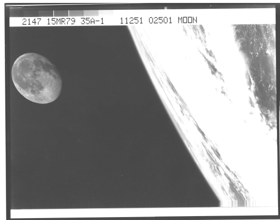
Figure 8.10: A visible GOES image containing both the Earth and the Moon. Note that the non-cloudy areas of the Earth are close in brightness to the Moon.
