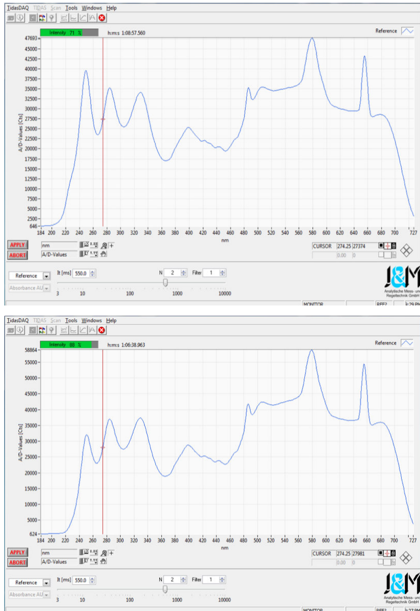
Figure 12. Raw (uncalibrated) intensity spectra of (a) ultrapure water and (b) 40 parts per thousand (ppt) sodium chloride (NaCl) solution from an UltraPath UPUV system with TIDAS diode-array spectrometer in real-time monitoring mode using TidasDAQ software provided by WPI.
