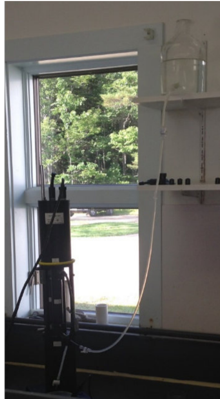
Figure 33. Photo of the instrument setup for the ac-s and ac-9 Sea-Bird Scientific absorption-attenuation (ac) meters used in the CDOM absorption round robins.
