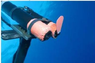
Copper tape on the instruments' housings and bio-shutter (Satlantic Hyperspectral radiometers)
