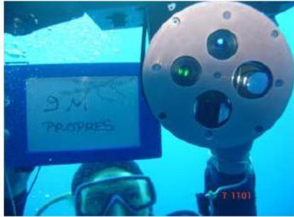
Copper face plate of the Hobilabs' Hydrosat-2 backscattering meter
