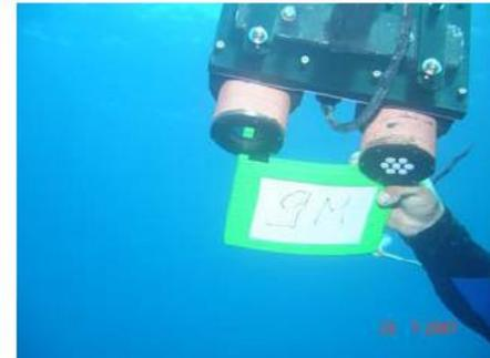
Copper tape on the instruments' housings for the Satlantic 7-band OCR-OCI/200 radiometers
