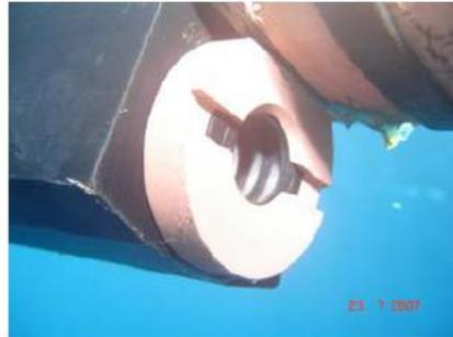
Copper rings around the emission and reception windows of the Wetlabs C-star beam transmissometers
