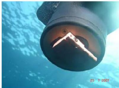
Copper face plate and copper shutter including a wiper for the Wetlabs Eco-FLNTU fluorometers (shutter closed)
