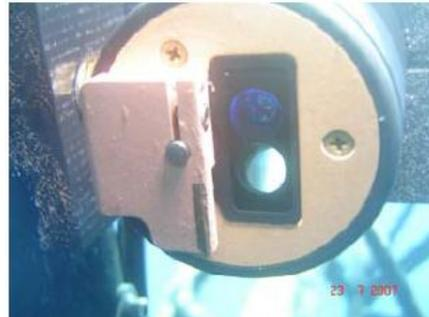
Copper face plate and copper shutter including a wiper for the Wetlabs Eco-FLNTU fluorometers (shutter opened, measuring)
