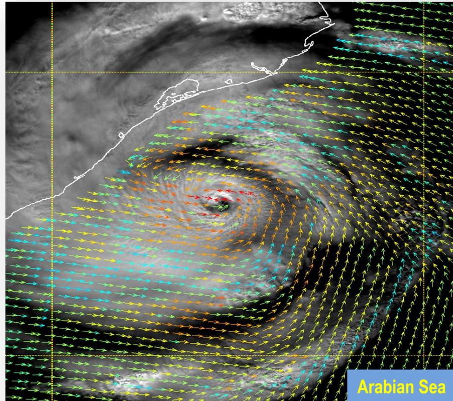
OCEANSAT-2 OCM B1 360 m Image overlaid by OCEANSAT-2 Scatterometer 12.5 Km Wind Vector. The image shows high speed winds at the eye of the cyclone and dissipated energy at the outer parts. As the cyclone settles down, the churning of oceanic water caused by it makes various parts of the region fertile and allows significant phytoplankton succession.
