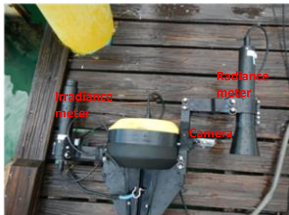
Figure 2. Design and configuration of a prototype radiometric package equipped with SBA. A sonar component for bottom depth is outside of the picture.
