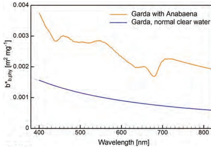
**Figure 6.2** Specific backscattering coefficients of phytoplankton in Lake Garda used for the simulations (CEOS 2018). Blue line — green algae from normal clear water; orange line — water with the cyanobacteria *Anabaena* sp. (both spectra provided by C. Giardino, personal communication).
