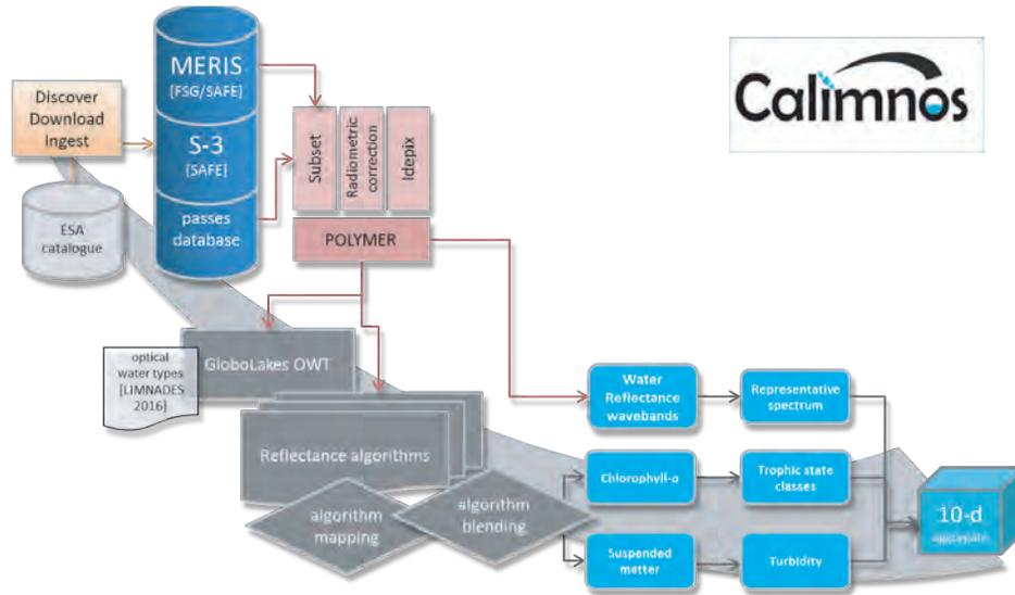
**Figure 7.3** Data flow from satellite data through to final products in the Copernicus Global Land project using the Calimnos processing chain (version 1.2, December 2017). S-3 = Sentinel-3 OLCI, OWT = optical water type classifier. Figure courtesy of Stefan Simis, Plymouth Marine Laboratory, UK.
