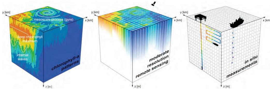
**Figure 3.6** Schematic surface and near-surface spatial structures in ambient waters (left) and typical sampling patterns using remote sensing (centre) and *in situ* measurement platforms (right). Figure from Odermatt et al. (2018) available under Creative Commons license.
