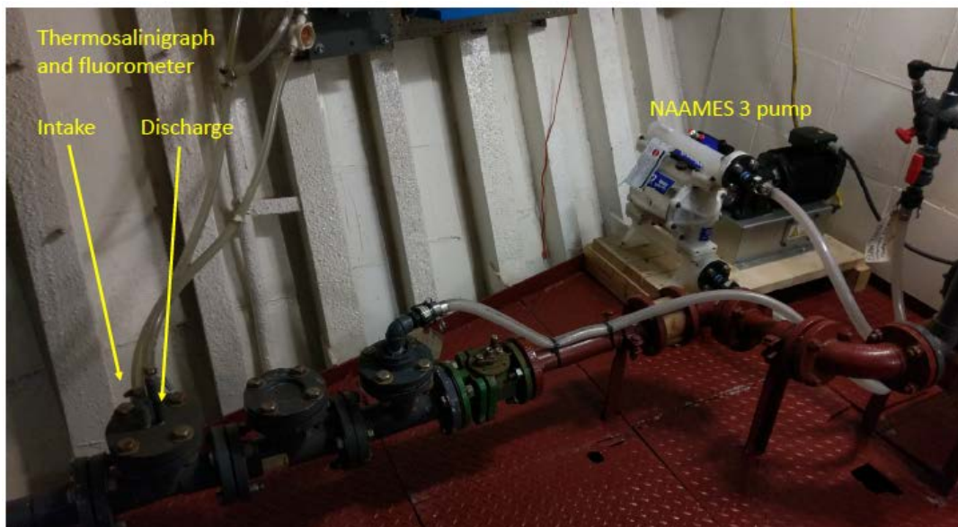
Figure 6. Underway instrument loop and pump on the R/V Atlantis during NAAMES03.
