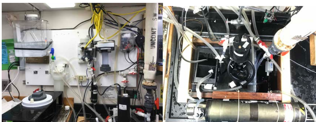
Figure 7. Front (left) and top (right) views of the sink on the R/V Atlantis where the inline system was set up. The water carboy on the left side was used for daily calibrations. In the sink there are a bb-box and the ac-S sitting in a plastic bin with ambient waters. The LISST is on the edge of the sink. The long white tube from the roof is the source of seawater which is routed through the debubbler. From there water flow into the automated switch (connected with yellow power/control cable) and from there to the instrument either through the 0.2 \mu m filter or unfiltered.
