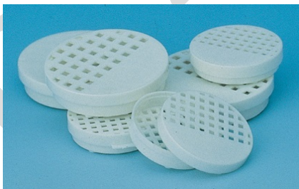
Figure 5.3. Example of plastic capsules for storing individual sample filters in liquid nitrogen.
