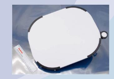
Solar Diffuser (SD): Spectralon<sup>®</sup> plate provides radiometric ref. measurements for the 14 VIIRS RSB bands.
