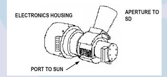
Solar Diffuser Stability Monitor (SDSM):
