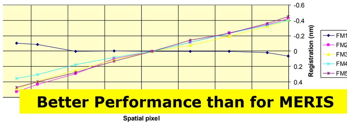
**OL-DE-020:** The spectral misregistration shall be less than 0.0014  $\mu\text{m}$  (goal: 0.001  $\mu\text{m}$ )
