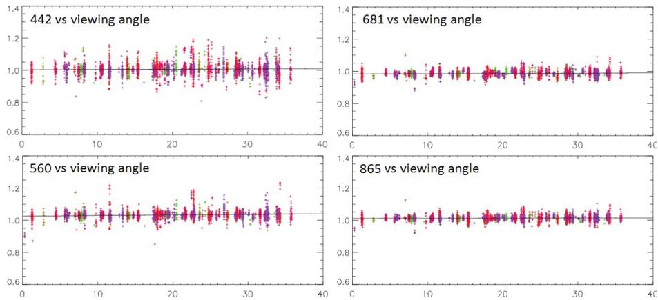
**Figure 4.9** Cross-calibration of MERIS and MODIS instruments in the 442, 560, 681, and 865 nm MERIS spectral bands as a function of the zenith viewing angle. Measurements are MERIS acquisitions from May to December 2009 and reference data are MODIS acquisitions from April to May 2011.
