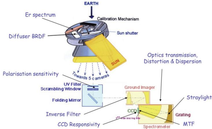
Figure 3.7 Diagram of the MERIS onboard calibration hardware.
