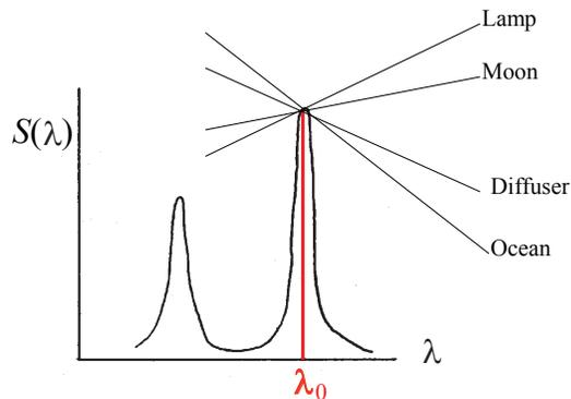
**Figure 2.4** Schematic showing how various sources all having the same radiance at  $\lambda_0$  but different spectral distributions would produce considerably different measured radiance  $\langle L \rangle_S$ .
