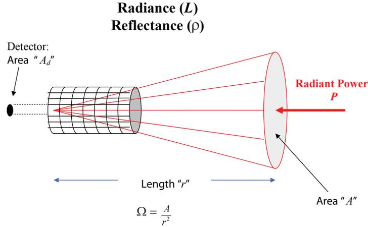
**Figure 2.1** Schematic of a radiometer. A detector of area  $A_d$  (sensitive only to radiation in a small band of wavelengths  $\lambda \pm \lambda/2$  around a central wavelength  $\lambda$ ) is allowed to view a scene with a field of view that is restricted to the solid angle  $\Omega$ . The tube restricting the field of view of the detector in the schematic is usually referred to as a *Gershun tube*.
