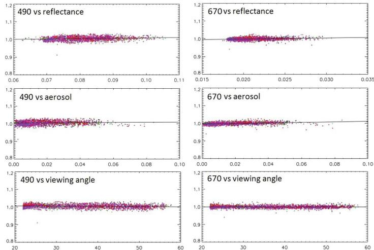
**Figure 4.3** Absolute radiometric calibration of SeaWiFS at 490 nm and 670 nm during the period from April to August 2000. Calibration coefficients  $\Delta A_k$  are displayed as a function of reflectance, aerosol optical thickness and zenith viewing angle.
