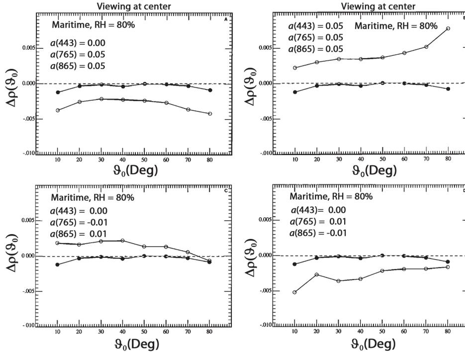
**Figure 2.13** The error in the retrieved  $t_v(443)\rho_w(443)$  for various calibration errors (from Gordon, 1997). In these simulations the aerosol optical depth at 865 nm was 0.2 and the Maritime model for a relative humidity of 80% was used to characterize the aerosol scattering.
