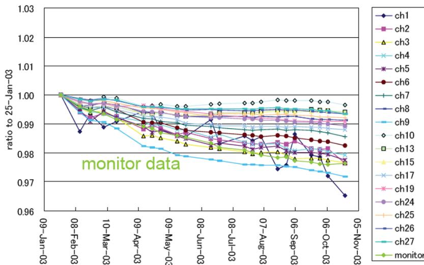
**Figure 3.3** Change in the responsivity (inverse of gain) of the Global Imager (GLI) spectral bands in the ultraviolet, visible, and near infrared, scan mirror B, from January to November 2003, as determined by internal lamp calibration (after Yoshida et al., 2004.)
