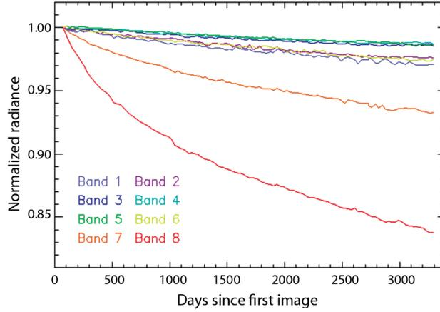
**Figure 3.6** Same data as in Figure 3.4 after correcting for the true variability of the lunar irradiance as calculated by the ROLO model (and after correction for over-sampling, an effect on the order of about 1% for SeaWiFS).
