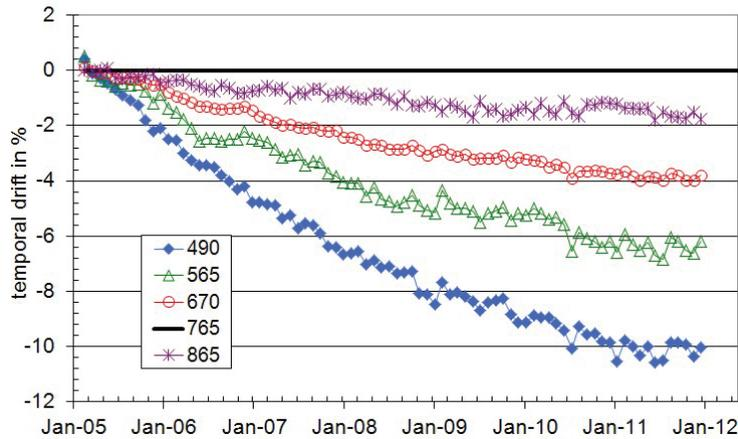
**Figure 4.8** Temporal monitoring of the radiometric sensitivity obtained for PARASOL/POLDER-3 spectral bands (except 443 nm) using the inter-band calibration over cloud method and 765 nm as a temporal stable reference (see also Fougnie and Bach, 2009).
