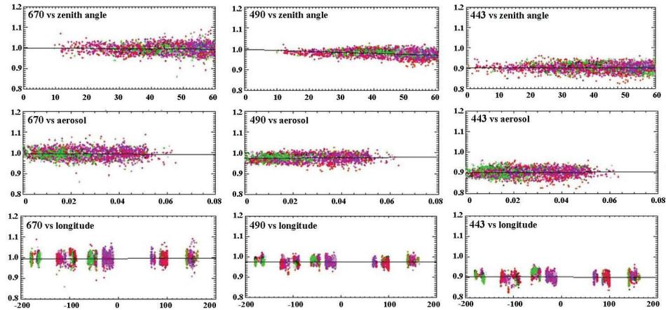
**Figure 4.2** Absolute radiometric calibration of POLDER-2 at 443, 490, and 670 nm during the period from January to June 2003. Calibration coefficients  $\Delta A_k$  are displayed as a function of viewing zenith angle (top), aerosol optical thickness (middle), and longitude (bottom).
