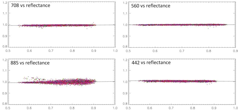
**Figure 4.7** Inter-band calibration ( $\Delta A_k$  coefficient) of the MERIS spectral bands at 442, 560, 708, and 885 nm using the cloud method. Data were collected between 2002 and 2011. The spectral band of reference is centered at 681 nm.
