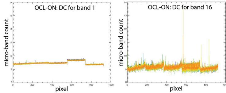
**Figure 3.10** Dark calibration measurements as a function of spatial pixel for all orbits in OCL-ON setting for band 1 (left) and smear band (right), scaled to micro-band level. 215 orbits are plotted on top of each other.
