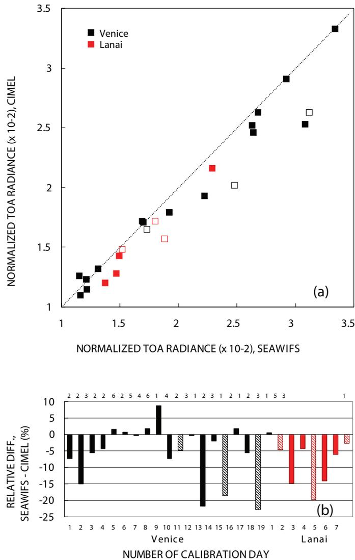
**Figure 4.13** SeaWiFS radiometric calibration in the near infrared (band 8), for the 19 days selected for the Venice site and the 7 days selected for the Lanai site. (a) CIMEL retrieved TOA radiance versus SeaWiFS TOA measurements. (b) Relative difference between SeaWiFS measurements and CIMEL retrievals. Labels on the top represent the number of principal plane sets used for the computation of the TOA radiance (after Martiny et al., 2005a).
