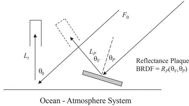
**Figure 2.2** Schematic describing the use of a reflectance plaque to effect on-orbit reflectance calibration of SeaWiFS and MODIS. The radiometer first views the ocean-atmosphere system and records a radiance  $L_t$ . It then views a reflectance plaque having a known bi-directional reflectance distribution function (BRDF) and measures a radiance  $L_p$ .
