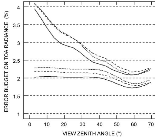
**Figure 4.12** Error budget for  $L_{TOA}$  computed for the M90 model (solid line), the T90 model (dashed line), and the U90 model (micro-dashed line). The visibility is 23 km, the solar zenith angle  $30^\circ$  (upper plots) and  $60^\circ$  (lower plots), the relative azimuth angle  $90^\circ$ , and the wind speed  $7 \text{ m s}^{-1}$ .
