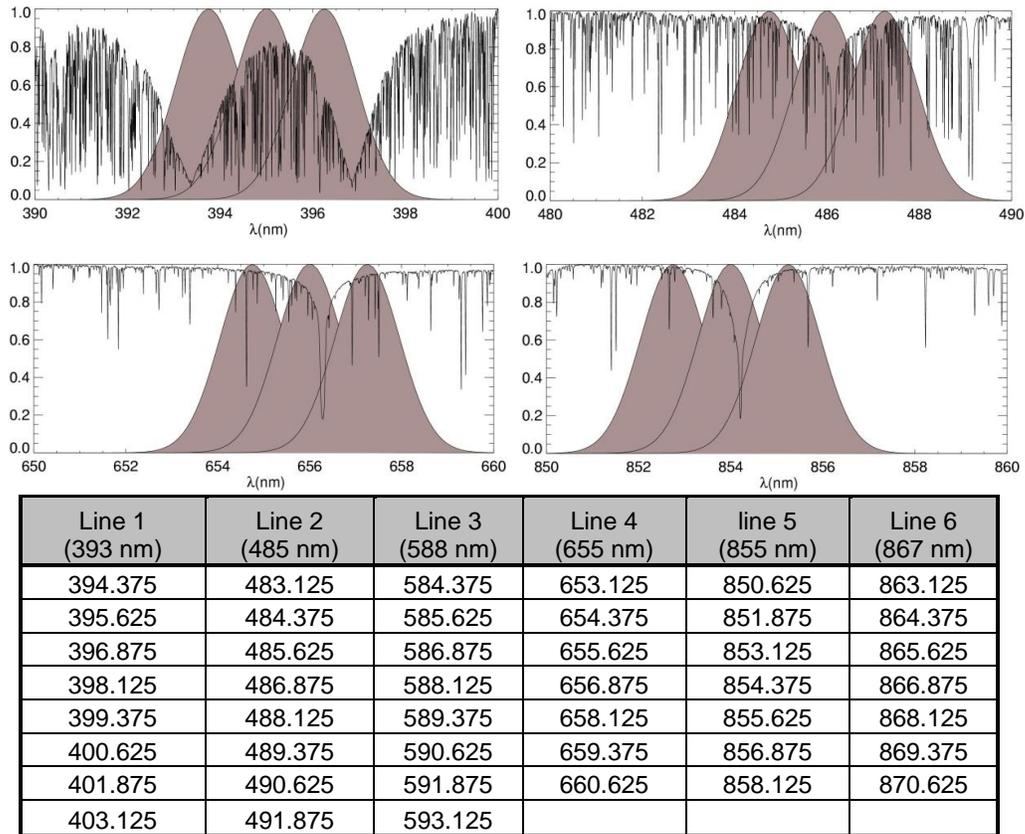
**Figure 3.14** Top: Fraunhofer spectrum with typical MERIS detector normalised spectral response function overlay; for lines 1, 2 4 and 5 (from left to right). Bottom: Instrument band configuration for Fraunhofer spectral calibration of MERIS.
