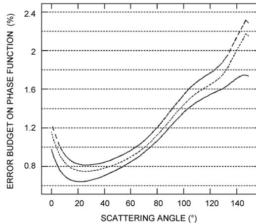
**Figure 4.11** Error budget for the  $\omega_a P_a$  product derived for the M90 model (solid line), the T90 model (dashed line), and the U90 model (micro-dashed line). The visibility is 23 km, the solar zenith angle  $75^\circ$ , the wind speed  $7 \text{ m s}^{-1}$  and the wavelength is 865 nm.
