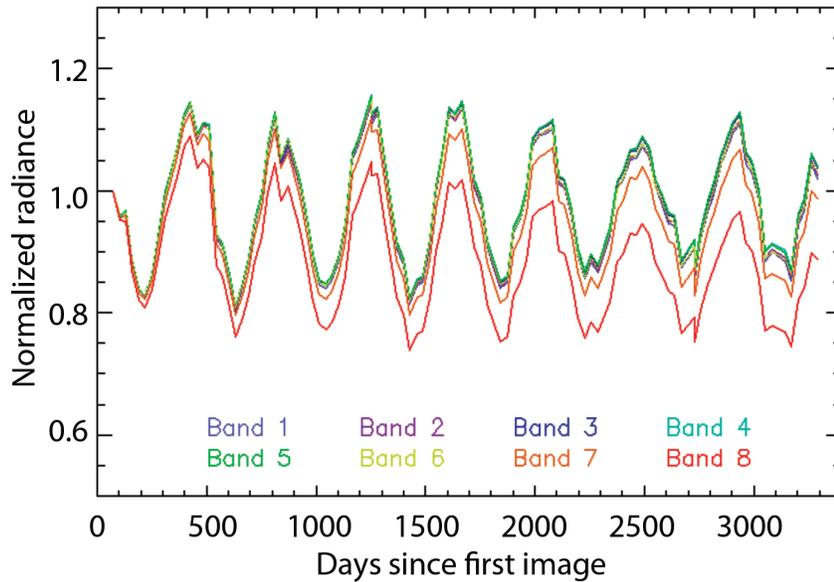
**Figure 3.4** Lunar irradiance as measured by SeaWiFS, plotted as radiance normalized to 1 for all bands at the first measurement (first 10 years of data). The data are dominated by the true variations of the lunar irradiance, even though the lunar phase angle is almost constant (about  $7^\circ$ ) for each measurement.
