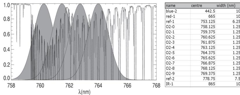
**Figure 3.13** Oxygen A-band absorption spectrum and instrument spectral band configuration for spectral calibration.
