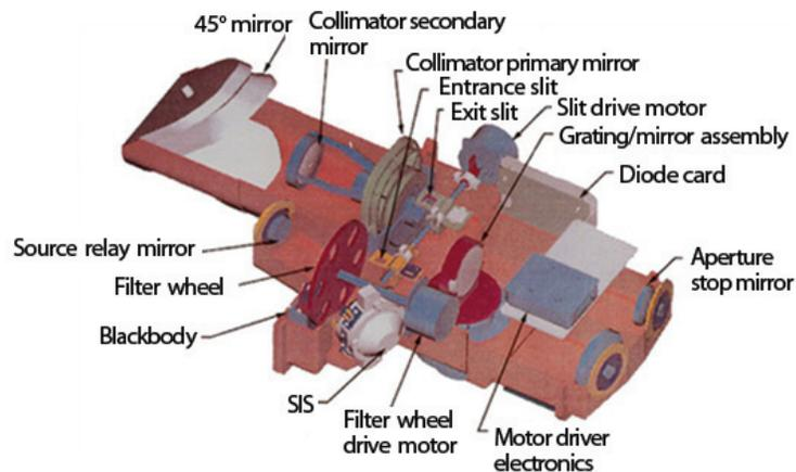
**Figure 3.11** MODIS Spectroradiometric Calibration Assembly (SRCA) (credit NASA).
