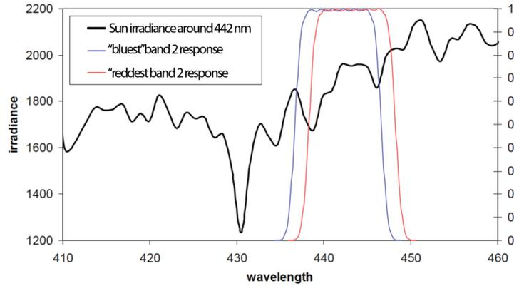
**Figure 3.15** Reference solar irradiance around 440 nm and the extreme spectral response functions of MERIS band 2 (for pixel 740 of camera 1 and pixel 1 of camera 2 as “bluest” and “reddest”, respectively).
