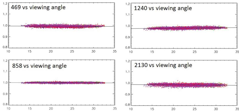
**Figure 4.5** Inter-band calibration ( $\Delta A_k$  coefficient) of the MODIS spectral bands at 469, 858, 1240, and 2130 nm using the sun glint method as a function of zenith viewing angle. Data were collected in December 2003. The spectral band of reference is centered at 645 nm.
