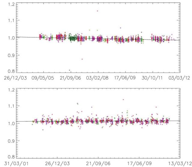
**Figure 4.6** Temporal evolution of the  $\Delta A_k$  coefficient obtained before correction at 765 nm for PARASOL (top) and after correction at 865 nm for MERIS (bottom) using the sun glint inter-band calibration method.
