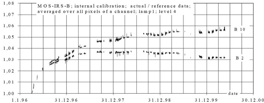
**Figure 3.2** Change in the gain of the Modular Optoelectronic Scanner (MOS) in spectral bands 2 and 10 during the period from April 1996 to December 2000, as determined by internal lamp calibration (after Neumann, 2001.)
